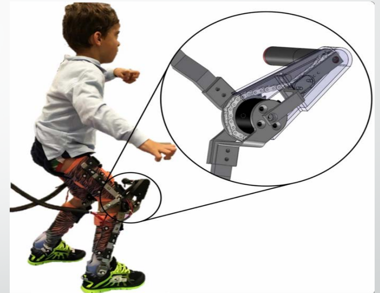
Figure 1: Adjustable Human-Exoskeleton Mounting Interface
